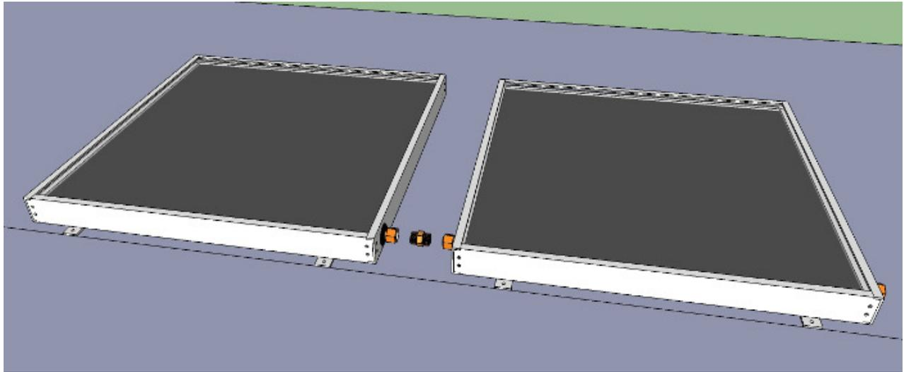
Start threading the union into the nuts on one panel and hand tighten only to allow some flexibility when lining up the panels. Bring the panels close to each other so the nuts on the second panel can be threaded onto the union, hand tighten. Slightly tighten the nuts on both sides. Not much torque is needed to form a tight seal. Once all the panels are connected further tighten each nut by about 1 turn.
