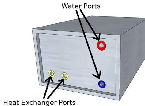
Install 2 of the 4 included 3/8" Compression to 1/2" Male NPT adapters into the heat exchanger ports.
