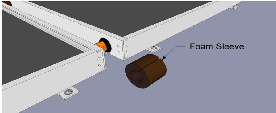
Install a foam sleeve over every fitting between panels as well as at the ends of the panel array.
