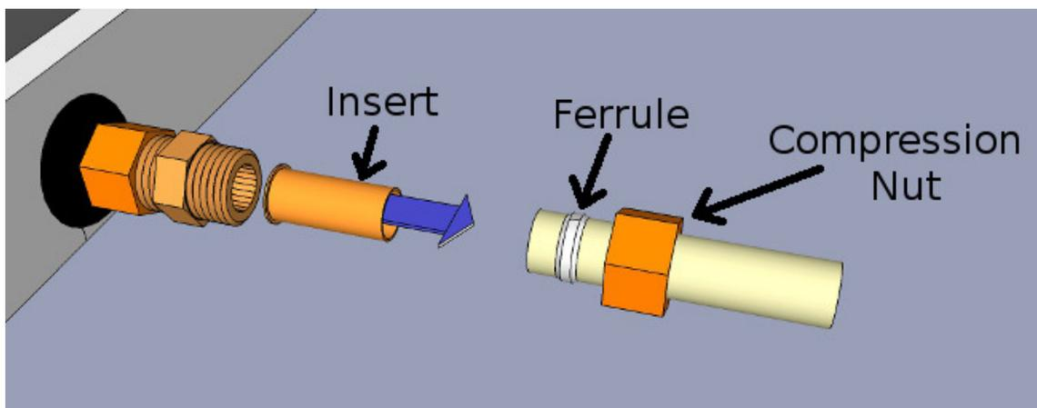
Finally push the tubes into the 3/8" compression unions and thread the compression nuts onto the union. Hand tighten and then tighten an additional turn.
