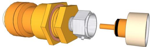
2. Manual bleed (open) – In this state the valve is open and will let air or water escape. When the top part of the valve is threaded halfway in the valve will be in this state.
