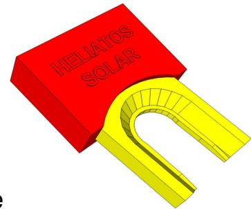
To unlock the fittings and remove them slide the tool onto the pipe so the lip in the yellow part is between the beige ring and the black rubber grommet.
