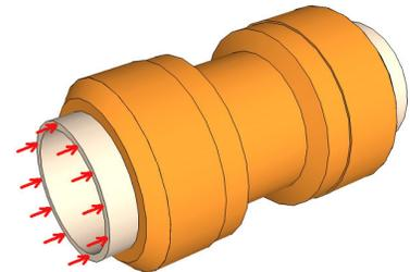
Pushing in this ring is not easy especially when the fittings are installed between two panles which is why we include a specially designed tool.
