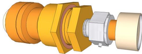
3. Automatic air only bleed – When the top of the valve is threaded all the way in and finger tight (DO NOT tighten with a wrench) the valve will allow air to escape but shuts off quickly once all the air is out of the system. A few drops of water might escape initially because the valve is operated by special hygroscopic discs getting wet and expanding.
