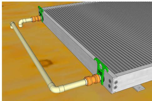
If you are using PEX tubing to connect to the panel array you need to put a plastic insert into the PEX tubing before you push it into the fitting. The plastic insert reinforces the PEX from the inside so that the push-fit fitting can hold on to the tubing securely.
