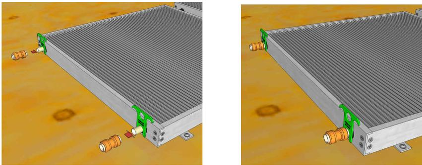
Next the connecting pipes can be pushed into the fittings. The proper insertion depth is close to 3/4". The spacers can be removed **AFTER** the pipes have been pushed in properly.
