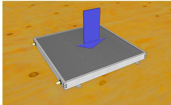
Each panel has to be securely tied down. This is especially true if it is mounted on a rack or on rails so that wind can catch the panels from below. We show a simple set of deck screws here, but depending what method you are planning to use you should follow the directions provided with your mounting hardware. Please remember that these panels are very light so that under no circumstances can you rely on their weight to hold them in place.
