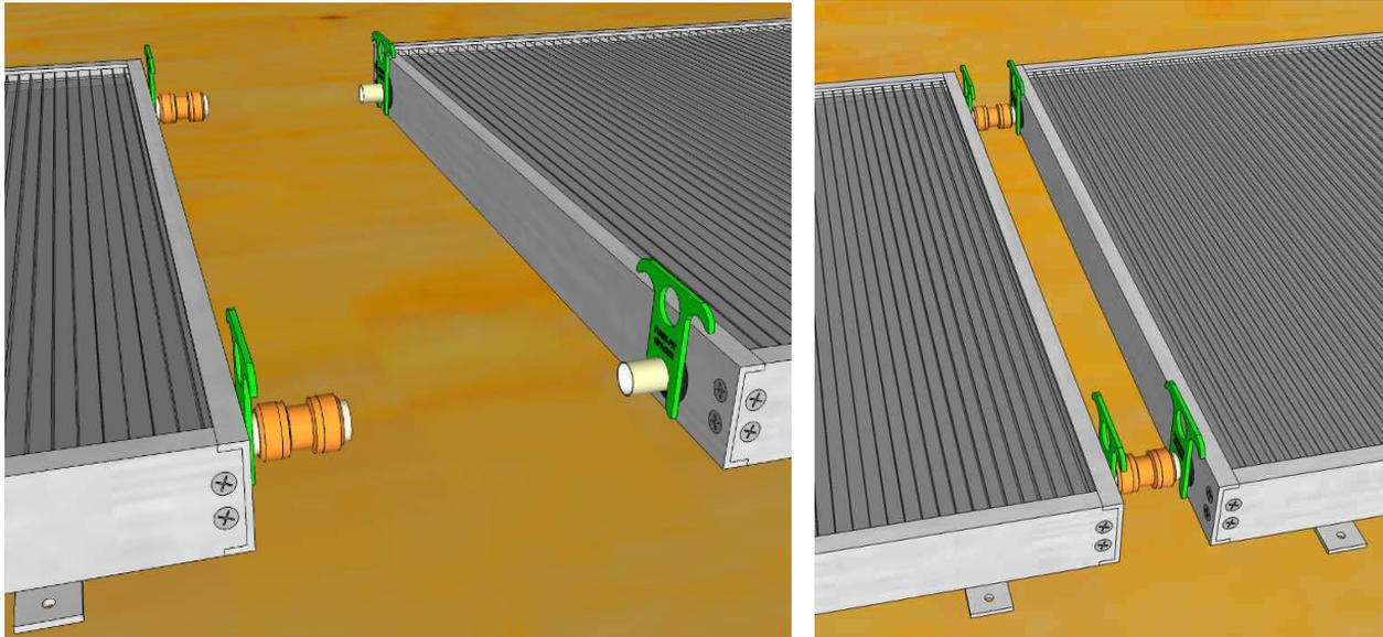
Once completely seated the fittings should be touching the spacers on both sides.
